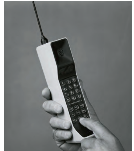
Fig. 6.3. The first mobile phone. It is the Motorola DynaTAC 8000X. It went on sale in 1983 at a price of $ 3,995. It had a weight of 0.79 kg and its battery took ten hours to charge. For its development, Motorola invested one hundred million dollars and its research lasted almost fifteen years.
